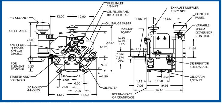
\* Net Weight Dry Standard Engine 410 lbs. (186.4 kg)
