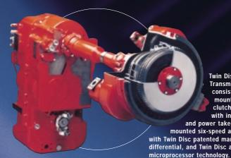
Twin Disc's Automatic Transmission System consists of an enginemounted modulated clutch torque converter with integral lock-up clutch and power take-off, independently mounted six-speed automatic transmission with Twin Disc patented managed biasing differential, and Twin Disc advanced
