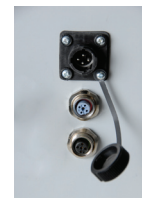
Top: CPC sealed dual float switch connector with cap Middle: M12 sealed transducer connector (cap not shown) Bottom: M12 sealed RS485 serial connector (cap not shown)
