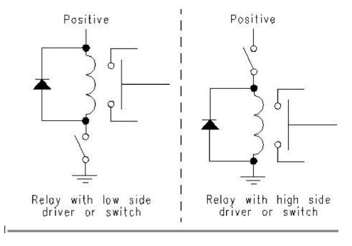
Relays and solenoids with built-in voltage transient suppression diodes are recommended whenever possible. Refer to the illustration for proper installation of diodes when built-in voltage transient suppression is not available.
