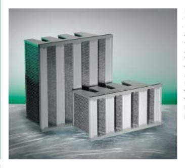
MANN+HUMMEL compact filter cells are proven in the fields of clean room technology, air-conditioning and ventilation systems, as well as in industrial processes. They are chemical adsorption filters suitable for use in technical applications to remove harmful gases and odours from the air. The core of the filter cells are activated carbon panels, as described on page 7. Depending on the requirements, MANN+HUMMEL offers its customers a wide range of media with or without impregnation.
