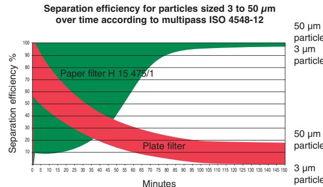
The separation efficiency of the paper filter increases during the life time of the filter.
