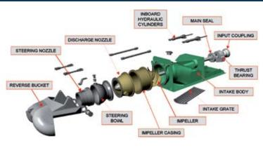
The **DOEN 200 Series** range of models can be matched to engines from 400kW to 4000kW. These high performance units are specially designed and built for continuous commercial use and to meet the exacting standards of marine classification societies. They can be installed as single or as multiple jets in fiberglass, aluminium or steel hulls. They can also be supplied as booster jets.
